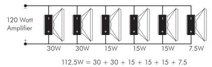
Amplifier power must be equal or higher than total power of all speakers
