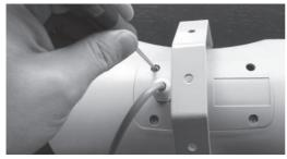
Remove the four screws from the top of the MPBD20-G
